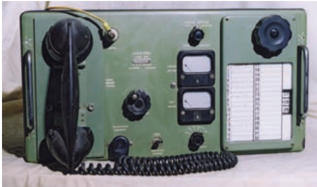
● Fig. 2: The Type 86D transmitter-receiver - also from Denmark. The drum with the channel selection numbers on the right holds the crystals within it (see text).
