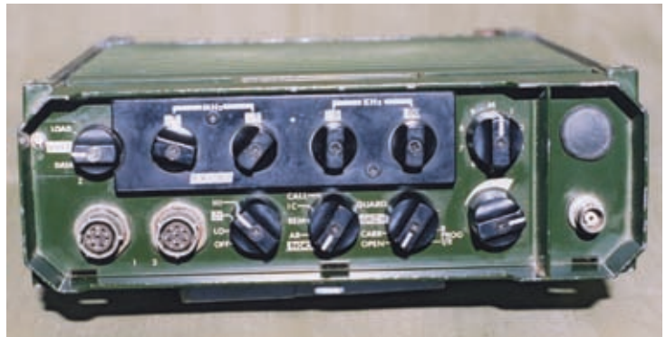
● Fig. 3: The Racal PRM4090 v.h.f. transceiver. It's provided with 'dial up' frequency selection, two handset sockets and the various other controls select memories and modes (see text).
