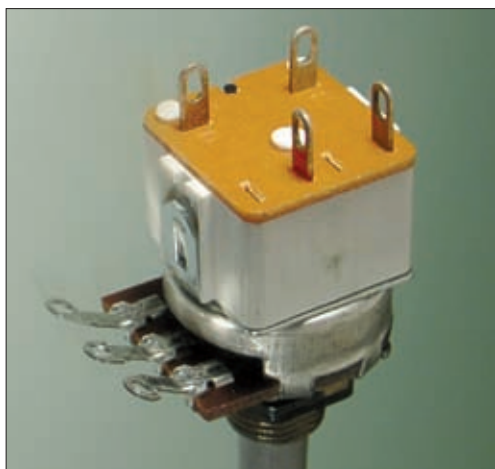
● Fig. 3: Combined variable resistor/potentiometer with DP On/Off switch (see text).
