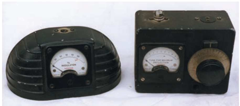
● Fig. 4: The two Eddystone measuring units, modulation depth meter on the left, field strength meter on the right (see text).
