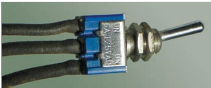
● Fig. 4: Subminiature SP C/O switch (see text).
