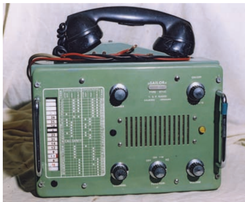
Fig. 1: The Danish 'Sailor' RT142 v.h.f. marine set, clean simple lines with the telephone type handset (see text).
